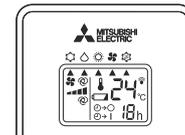
Press STOP/OPERATE (OFF/ON) button of the remote controller (the set temperature is displayed) with the remote controller headed towards the indoor unit. ※1
